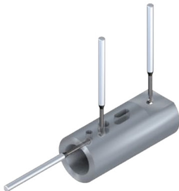
Deburring after drilling
