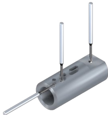
Deburring after drilling
