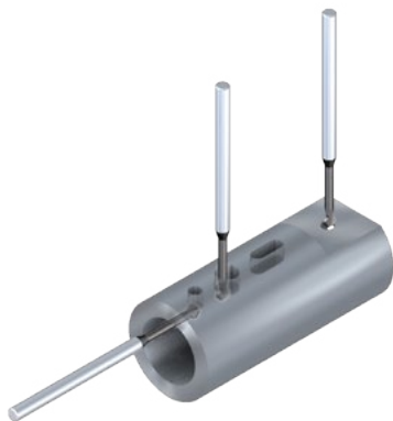
Deburring after drilling
