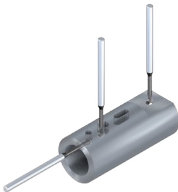
Deburring after drilling
