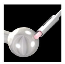
**Convex Surface:** One manufacturer deburred, removed cutter marks, and polished a cobalt chromium-alloy convex surface manually with grindstones and sandpaper, which made it difficult to control dimensional integrity and surface quality. With a Xebec Surface Brush, the manufacturer automated polishing and achieved stable and consistent quality in a shorter cycle time.
