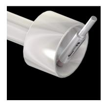
Medical Cup: A manufacturer used manual processes with grindstones and sandpaper to deburr, remove cutter marks and polish a cobalt-chromium alloy medical cup. This finish quality was unreliable and it was challenging to maintain shape. When they introduced the Xebec Surface Brush in their CNC machining process for polishing, they realized stable quality in a shorter cycle time.
