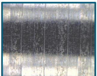
After Polishing with Xebec Surface roughness improved to = Ra 0.03 μm
